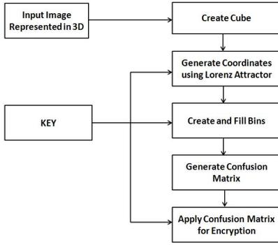
Fig. 1: Flow Chart of the Encryption Method
