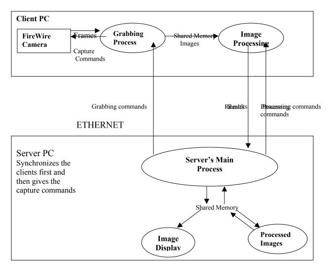
Process which issues the grabbing commands to the FireWire cameras and stores the results in a shared memory. Another process does image processing at the client and sends the processed images to the server.
